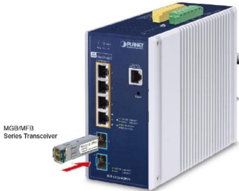
Figure 2-21: Plugging in the SFP/SFP+ Transceiver
